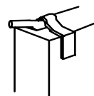
Type 8 - Horizontal metal peg fixed to top of headstock
